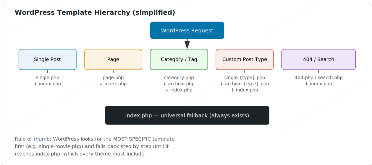
Fig 4.2 — Simplified Template Hierarchy showing fallback order per content type
